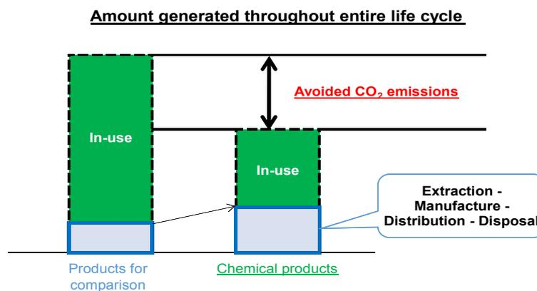
Fig. 19. Method of assessment using cLCA
