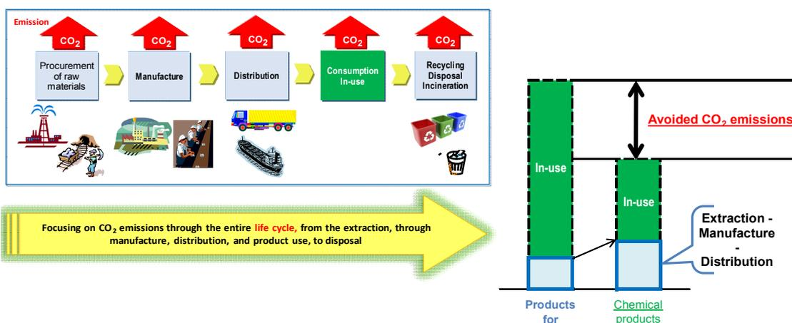
Fig. 7. Method of assessment using cLCA
