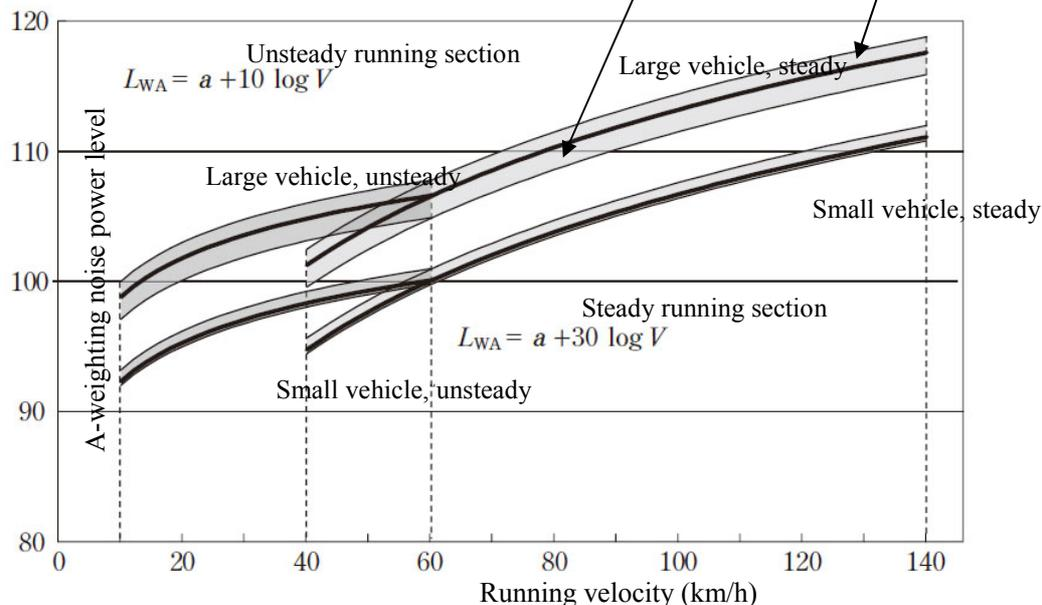
**Figure 2.13-A: Difference in noise power level and establishment of an uncertainty distribution of parameters**
