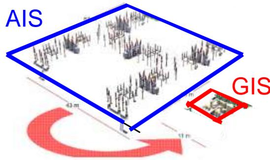
Figure 3.2-1 Image of downsizing of a substation
