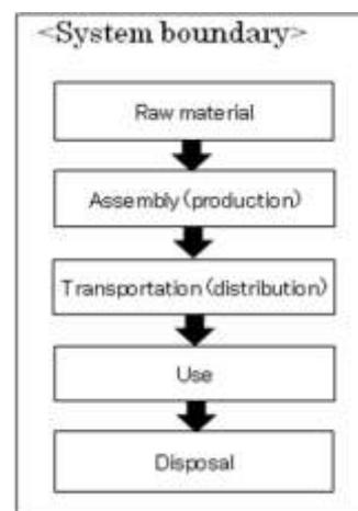
Figure 3.3-1 System boundary of LCD projector
