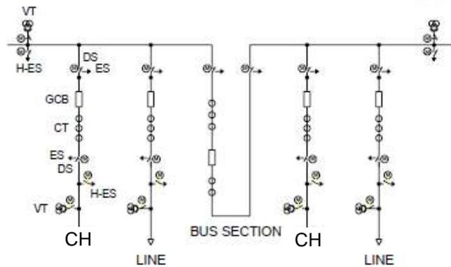
Figure 3.1-1 145kV switchgear single-line diagram
