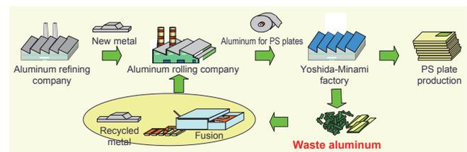
Figure 3 Closed loop recycling of cutting waste
