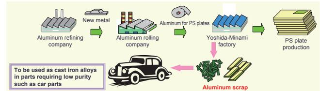
Figure 4 Conventional cutting waste recycling (cascade recycling)
