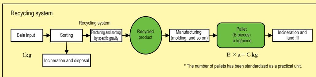
Figure 1: Material recycling (one-way pallet)
