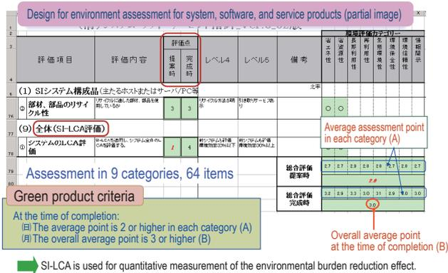
Figure 10 Assessment for Design for Environment for System Products (partial image)
