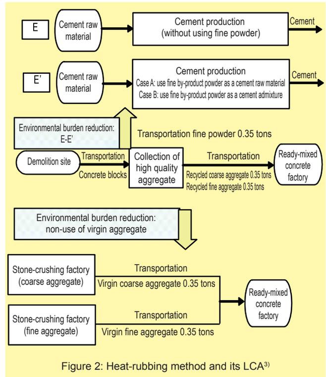
Figure 2: Heat-rubbing method and its LCA<sup>3)</sup>
