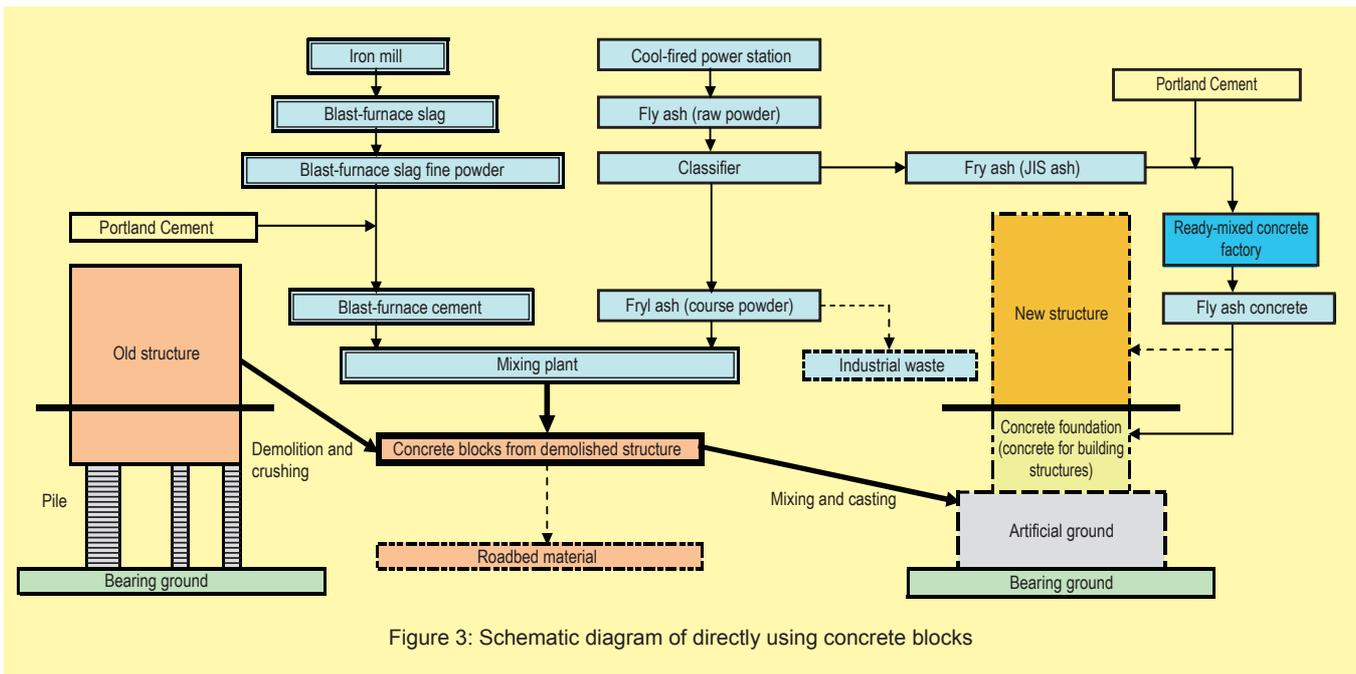
Figure 3: Schematic diagram of directly using concrete blocks
