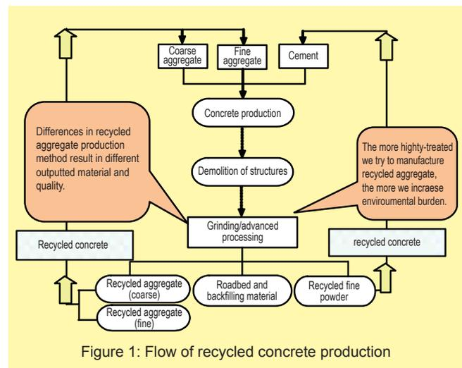
Figure 1: Flow of recycled concrete production
