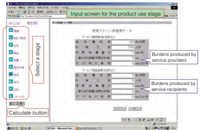
Figure 3 SI-LCA input interface (example)
