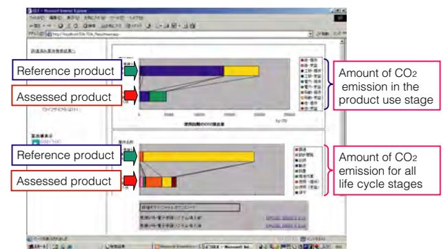
Figure 4 Example of the SI-LCA assessment result screen
