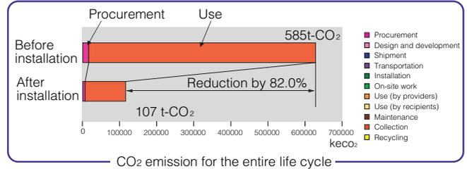
**Figure 7 Assessment results before and after the electronic form system installation**
